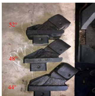
Fig. 11 Pick holders with different angles
