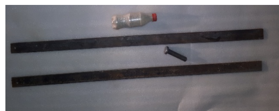
Fig. 4 The bottle filled with soil, two steel strips, and a stud
