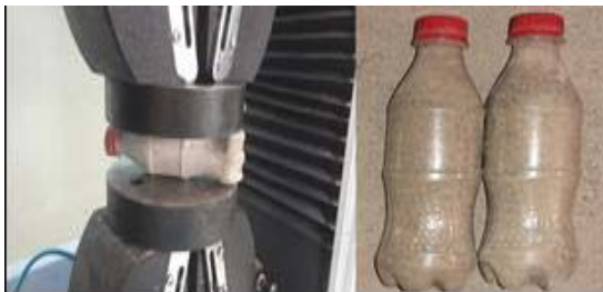
Fig. 2 The bottle filled with soil under compressive force in the pressure device and two bottles filled with soil
