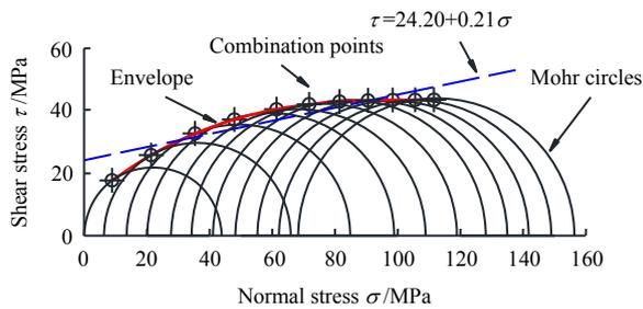
**Fig. 6 Shear strength envelope and Mohr's circles of Indiana limestone**
