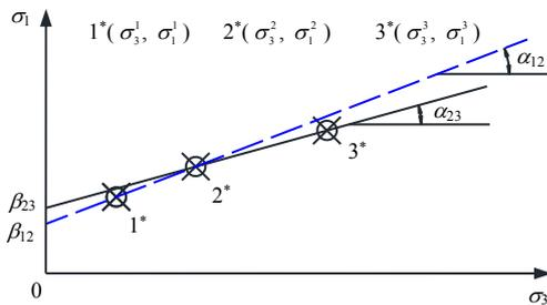
Fig. 3 LRM under the effect of confining pressure on the triaxial strength of rocks
