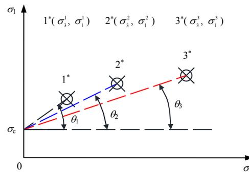
Fig. 4 Confining pressure effect of triaxial strength of rocks
