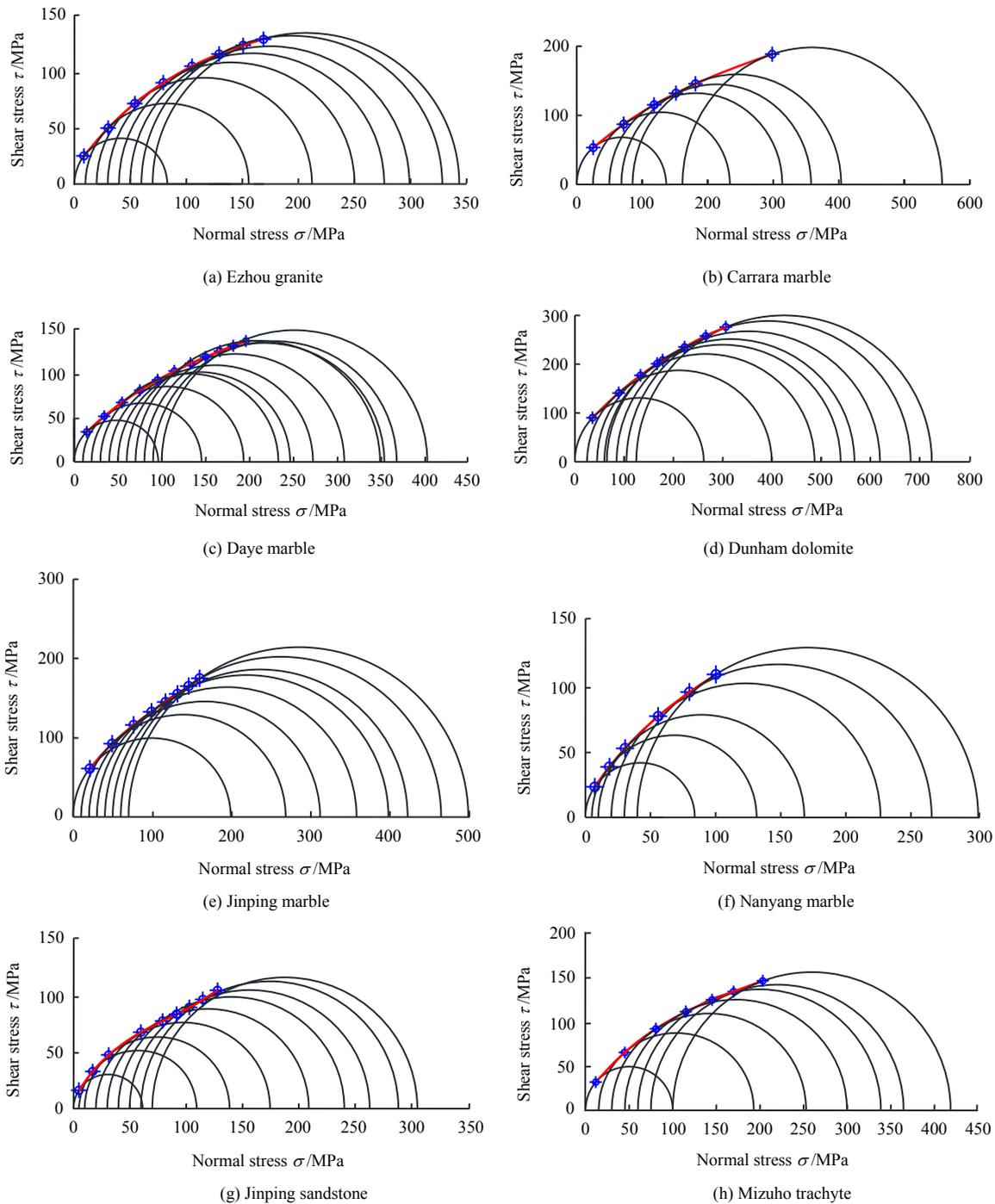
Fig. 7 Shear strength envelopes and Mohr's circles of eight types of rocks
