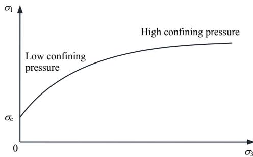
Fig. 2 Triaxial strength envelope of rocks
