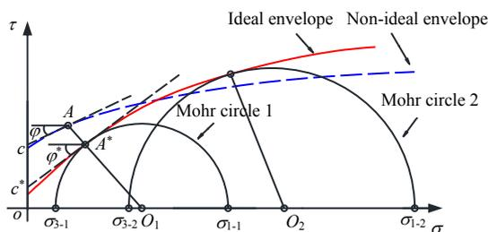
Fig. 5 Diagram of shear strength envelope
