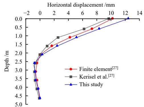
Fig. 7 Comparison curves of horizontal displacements of piles
