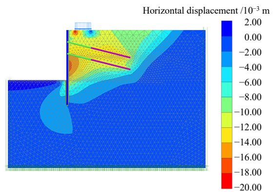
Fig. 10 Nephogram of overall horizontal displacements after excavation
