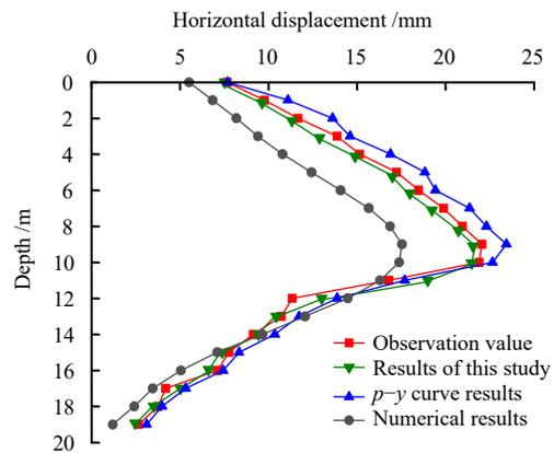
Fig. 11 Comparison curves of horizontal displacements of piles
