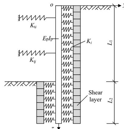
Fig. 3 Calculation diagram of pile–anchor retaining structure in two-parameter foundation model
