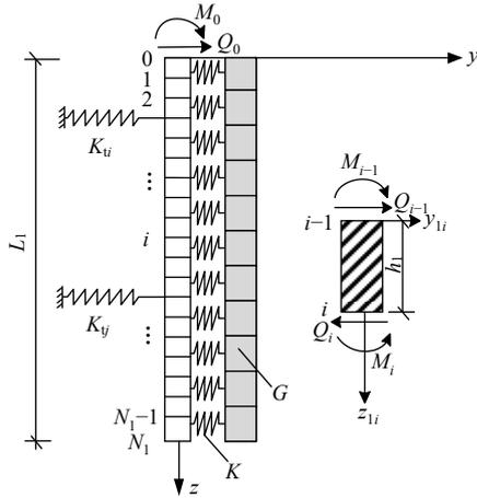
Fig. 4 Calculation diagram of the free section
