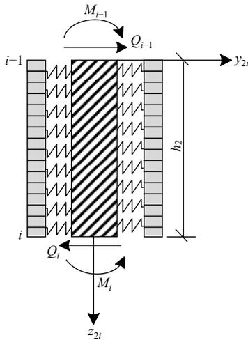
Fig. 5 Calculation diagram of the embedded section
