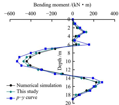
Fig. 12 Comparison curves of pile bending moments
