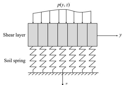
Fig. 1 Pasternak two-parameter foundation model
