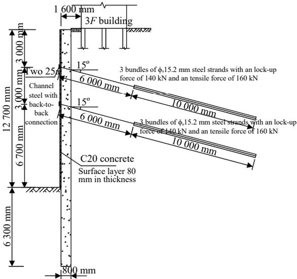
Fig. 8 Section of pile-anchor structure retaining scheme
