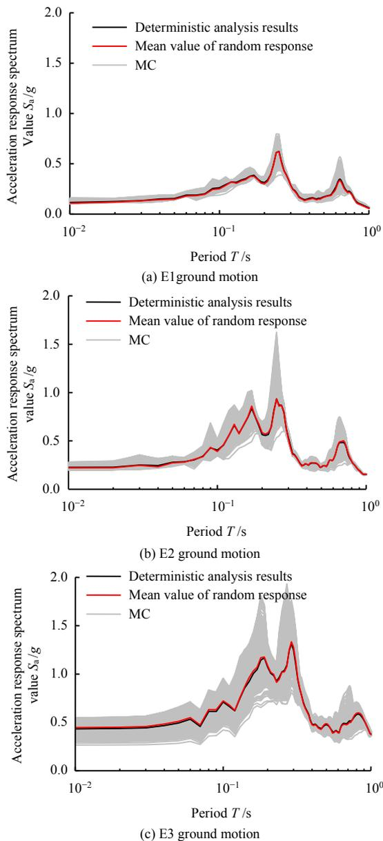
**Fig. 11 Comparison of acceleration response spectra at ground surface under E1, E2 and E3 ground motions**
