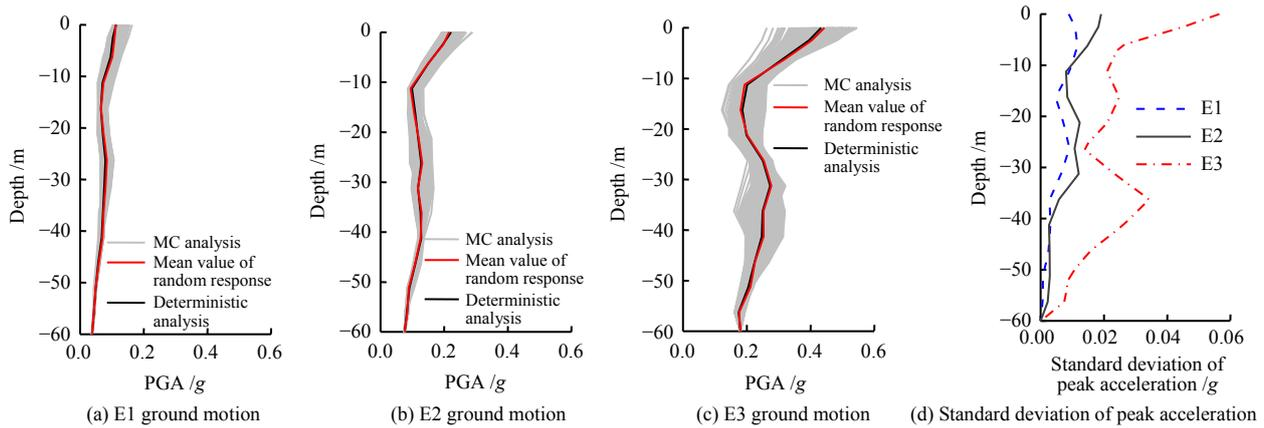
**Fig.9** Calculated results of site peak acceleration profile under ground motion of E1, E2 and E3
