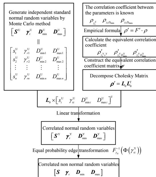
**Fig. 4 Flowchart of random sample generation considering the correlation among parameters**
