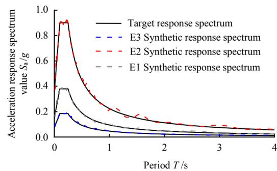
(a) Seismic acceleration response spectrum of class  $I_0$  site under different recurrence periods
