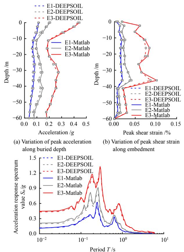
**Fig. 3 Comparison of calculation results between the developed program and DEEPSOIL**
