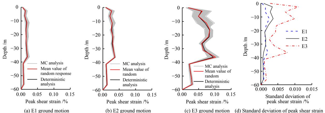
**Fig. 8 Calculated results of site peak shear strain profile under E1, E2 and E3 ground motions**
