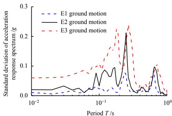
**Fig. 12 Standard deviations of surface acceleration response spectra under E1, E2 and E3 earthquakes**
