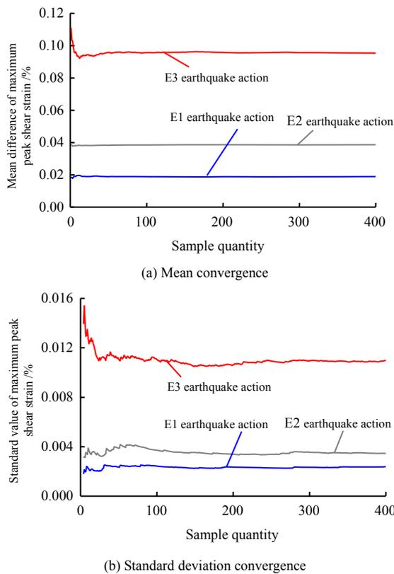
**Fig. 7 Convergence of mean and standard deviation of maximum peak shear strain of engineering site obtained from Monte Carlo Simulation method**
