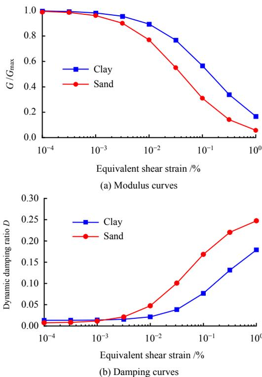
**Fig. 2 Dynamic shear modulus ratio and dynamic damping ratio of sand and clay**
