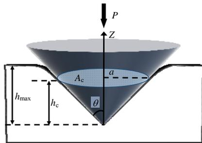
(a) Schematic diagram of nanoindentation
