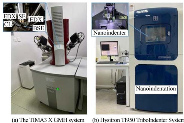
Fig. 1 Microscale rock mechanics experiment system(micro-RME)
