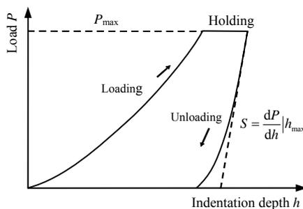
(b) Typical load-displacement curve
