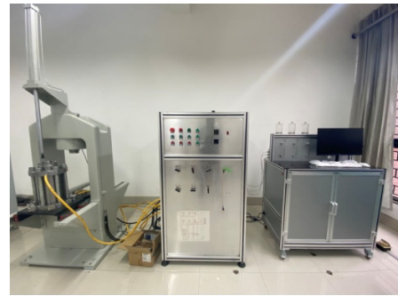
Fig. 1 Rock triaxial stress–seepage coupling test system
