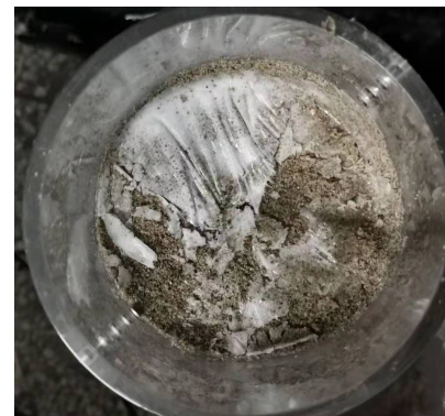
Fig. 14 Photo of frozen soil at cold end
