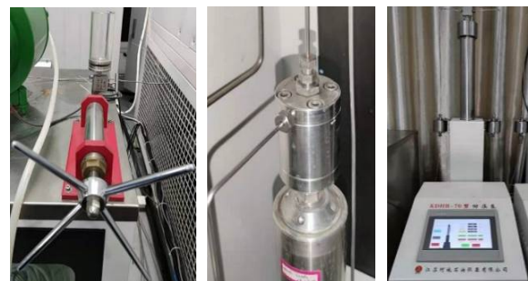
(a) Horizontal manual back pressure pump (b) Back pressure valve (c) Automatic back pressure pump
