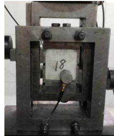
(c) Layout of the AE sensors
