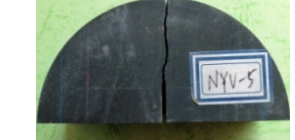
(d) The crack obtained by Zhao et al. [20]
