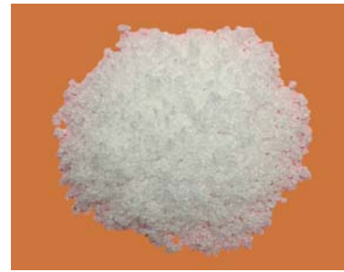
(a) Mixture of fused quartz, silica powder and mixed mineral oil
