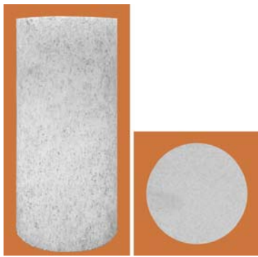
Fig. 3 Sample of the transparent cemented soil
