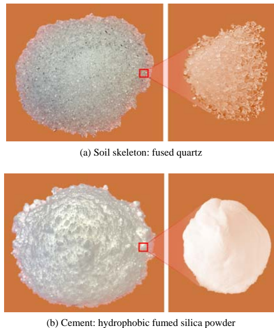
Fig. 1 Skeleton and cement of the transparent soil
