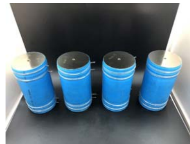
Fig. 3 Creep specimens after completion of sealing
