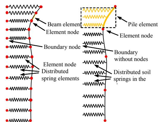
(a) Discrete spring element model (b) Pile element model
