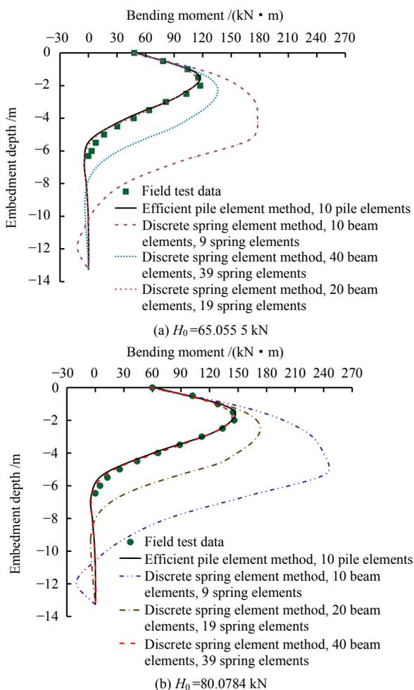
**Fig. 9** Depth–bending moment curves of pile
