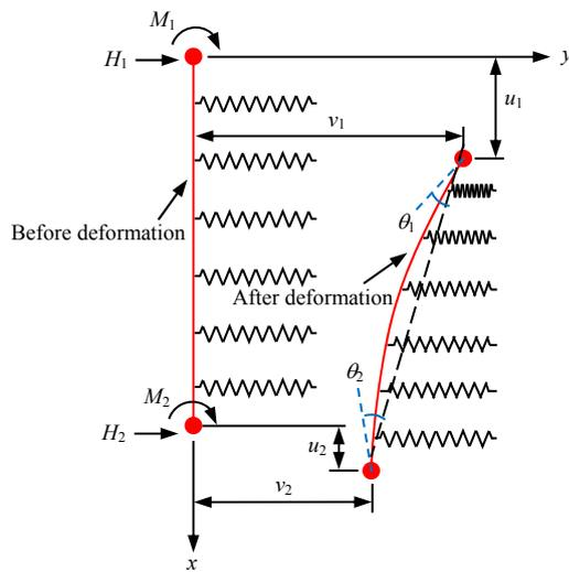
Fig. 3 Forces and deformations of pile element
