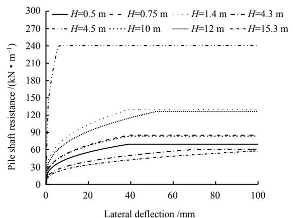
**Fig. 7 *p-y* curves of each soil layer**
