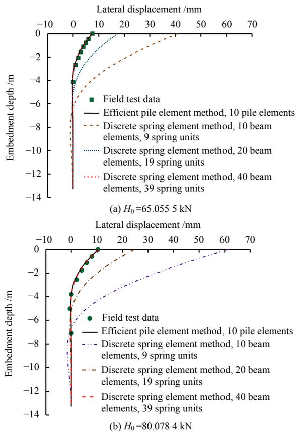
**Fig. 8** Depth–lateral displacement curves of pile
