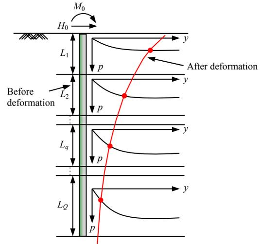
Fig. 4  $p$ - $y$  curves of each soil layer along the pile length
