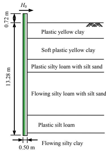
**Fig. 6 Geological profile of the test site**
