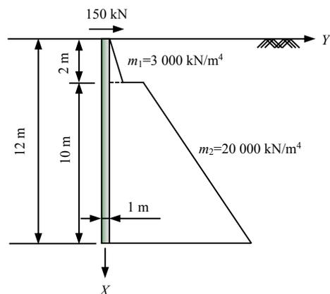
Fig. 5 Diagram of the pile–soil system
