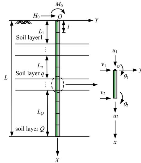
**Fig.2 Model of laterally-loaded pile in multi-layered soils**
