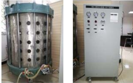
Fig. 2 YRK-2 rock immersion–air drying tester
