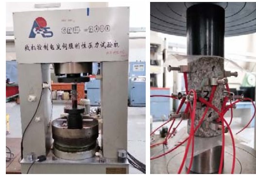
(a) Servo rigidity testing machine (b) Installation of sensors
