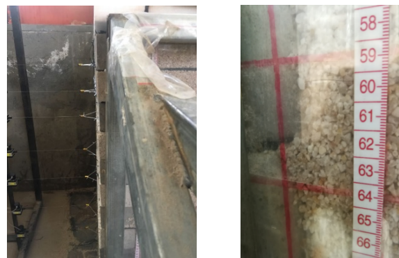
(a) Side wall of facing layer inclines outwards (b) Filling is squeezed into side wall block
