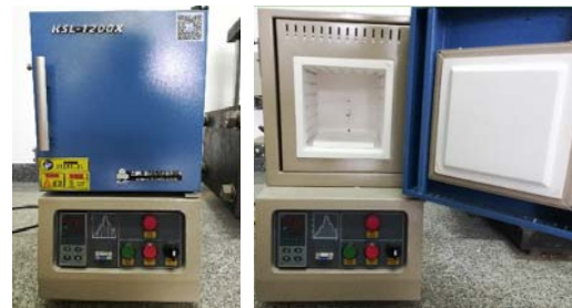
Fig. 2 KSL-1200X-J box resistance furnace
