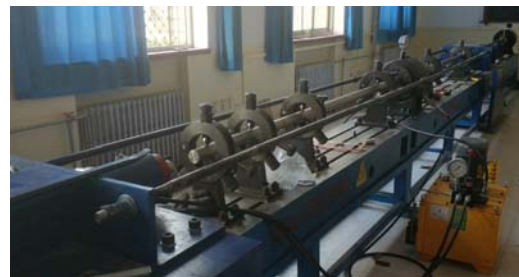
Fig. 2 SHPB test equipment
