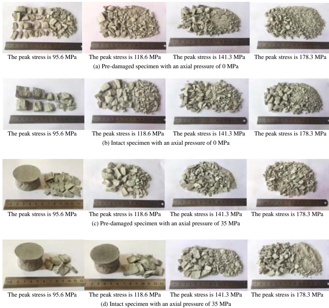
Fig. 8 Photos of damaged samples under different incident waves
