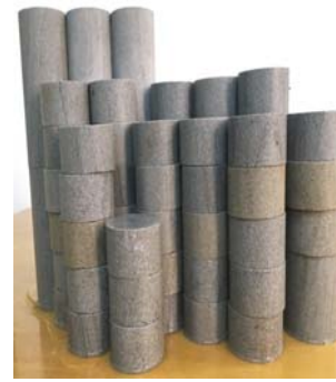
Fig. 1 Samples of grey sandstone for tests
