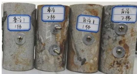
**Fig. 10 Sandstone specimens anchored by one or two bolts**
