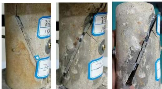
**Fig. 14 Failure mode of sandstone specimens with prestressed bolt–grouting reinforcement**
