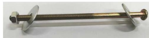
Fig. 6 Bolt for simulating the anchor rod
