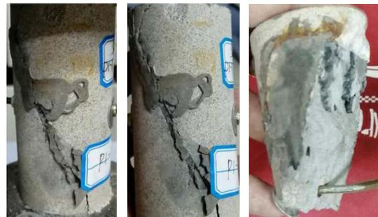
**Fig. 12 Failure mode of sandstone specimens with ordinary bolt-grouting reinforcement**
