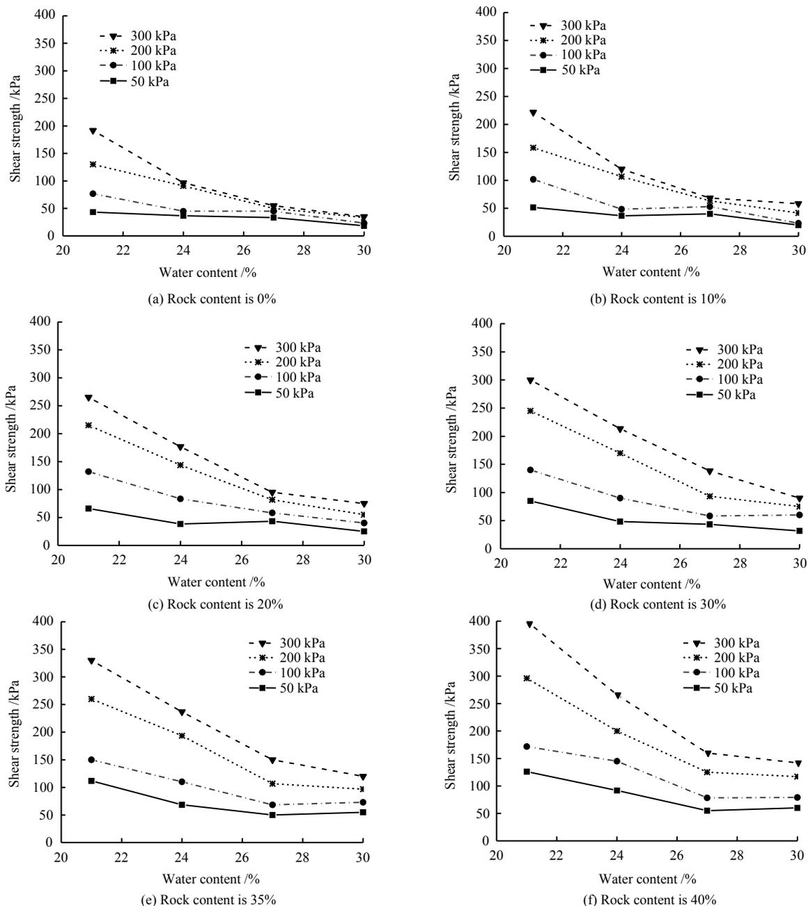
Fig. 3 Changing rule of shear strength of freezing-thawing interface under the influence of water content
