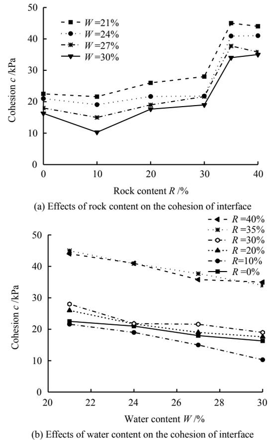
Fig. 5 Effects of water content and rock content on the cohesion of interface
