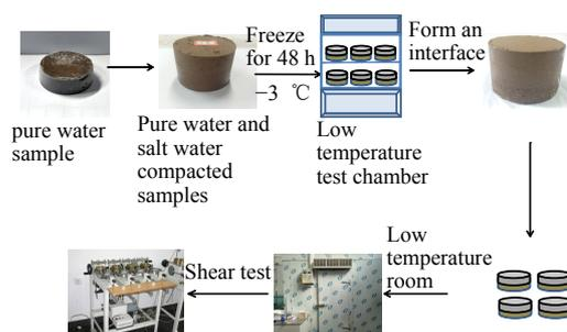
Fig. 2 Test procedure diagram of freezing-thawing interface of soil-rock mixture
