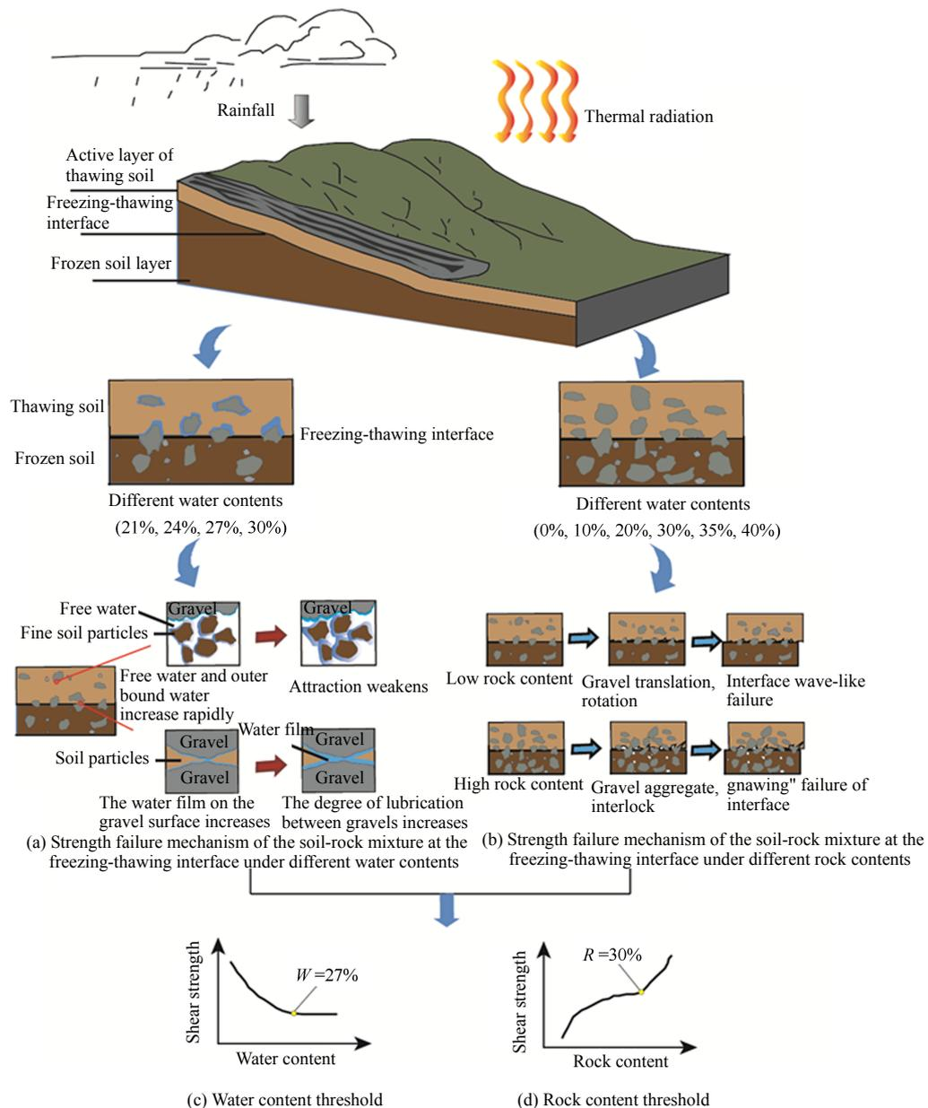
Fig. 7 Schematic diagram of the landslide mechanism of soil-rock mixture in the permafrost region
