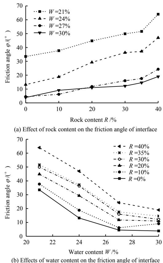
Fig. 6 Effects of water content and rock content on the friction angle of interface
