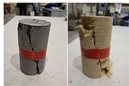
(a) Uniaxial compression test (left: rock-like material, right: sandstone)
