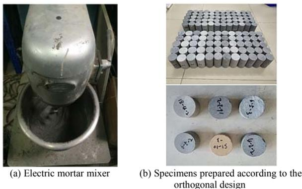
**Fig. 1 Electric mortar mixer and specimens prepared according to the orthogonal design**
