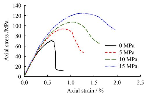
**Fig. 7 Stress–strain curves of the rock-like material under different confining stresses**
