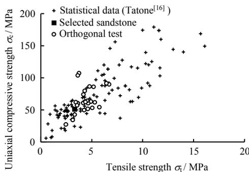
Fig.4 Comparison of the rock replica and natural sandstone based on the ratio of  $\sigma_c$  to  $\sigma_t$  (data from Tatone<sup>[16]</sup>)
