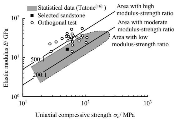
Fig.3 Comparison of the rock replica and natural sandstone based on the ratio of  $E$  to  $\sigma_c$  (data from Tatone<sup>[16]</sup>)
