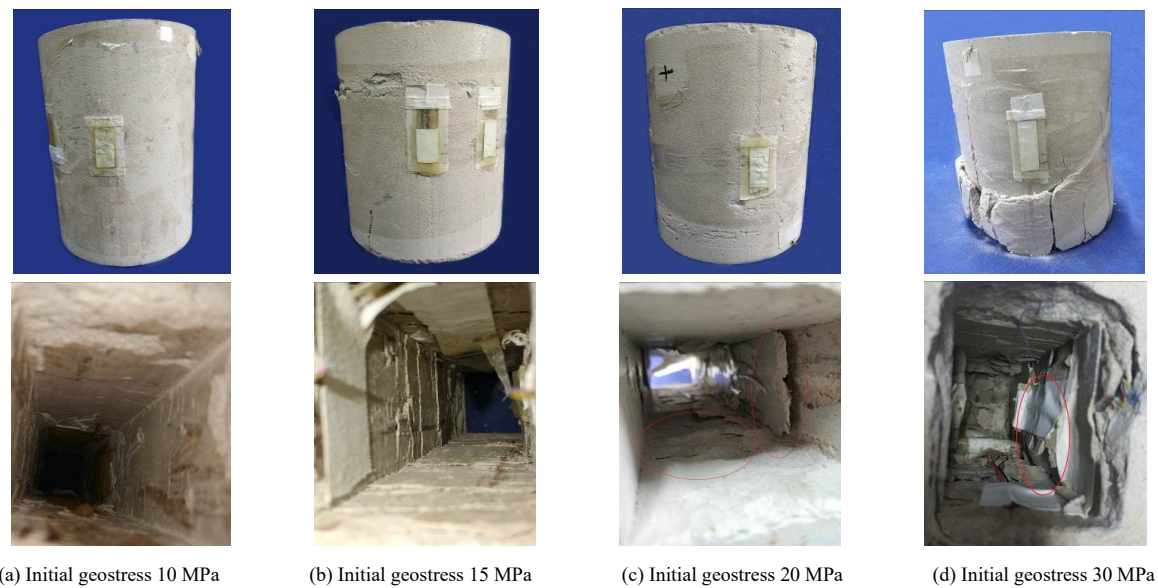
Fig. 11 Failure characteristics of specimens
