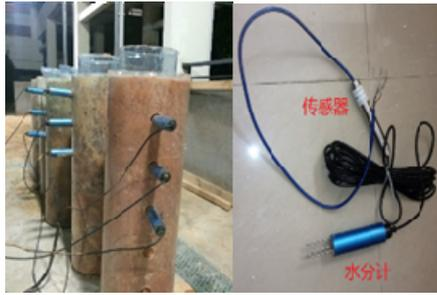
Fig.2 Soil column infiltration testing device
