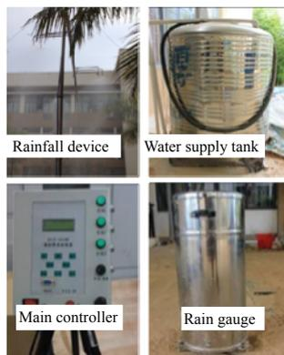
Fig.3 Main equipment of rainfall simulation
