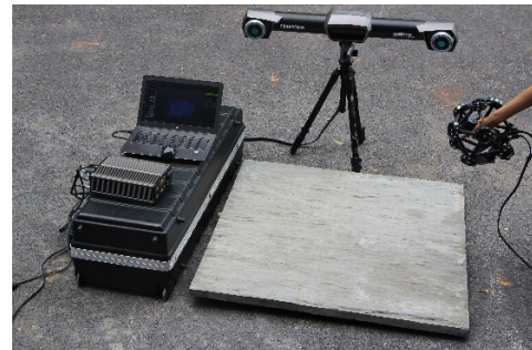
Fig.2 3D laser scanning of structural surface
