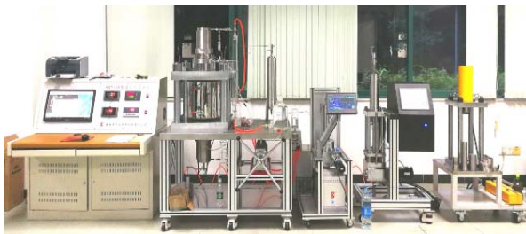
(a) Photo of the improved diagenesis system
