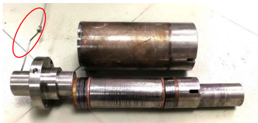
(b) Rock core mold and sealing device
