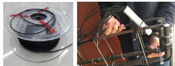
Fig.4 New type of tight sheathed strain sensing fiber
