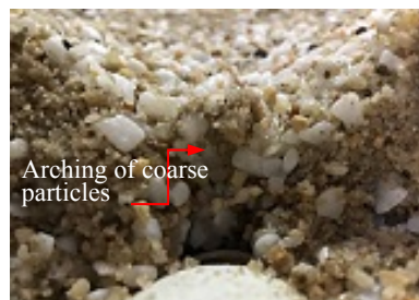
Fig.8 Arching photo of coarse particles above the damaged mouth
