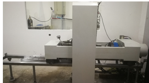
Fig.1 Shear-seepage coupled test system for rock joints
