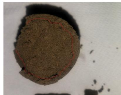
(a) Circumferential erosion channel
