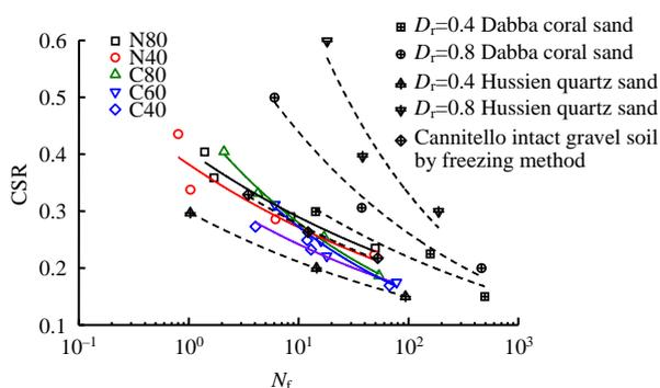
Fig. 5 CSR– $N_f$  relationship curves of silica sands and coralline soils with different relative densities
