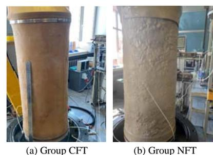
Fig. 2 Typical sample appearance of different sample groups
