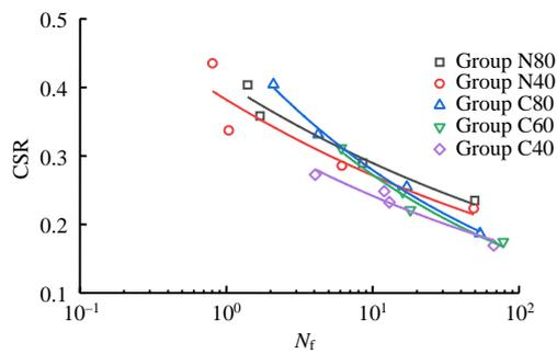
Fig. 4 CSR- $N_f$  relationship curves of CFT and NFT sample groups
