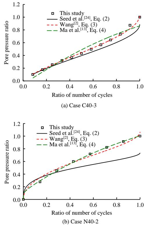
Fig. 6 Typical results of fitting analysis of the relationship between pore pressure ratio and ratio of number of cycles
