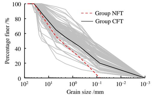
Fig. 1 Grain size distributions of the in situ and representative samples
