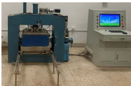
Fig. 2 Diagram of large-scale temperature-controlled submerged direct shear apparatus
