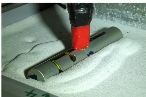
Fig. 4 Pipe penetration process
