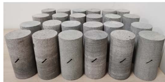
(a) Sandstone specimen with prefabricated crack
