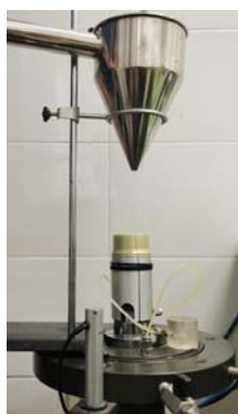
Fig. 3 Sample preparation with sand pluviation method
