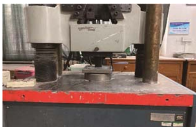
(a) WAW31000 microcomputer servo universal testing machine
