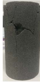
(a) Failure mode of PT samples
