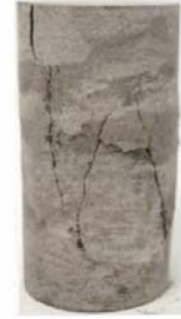
(b) Failure mode of weakly cemented coarse-grained sandstone [25]
