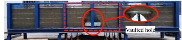
(b) Soil deformation after the 2 nd step of adjustment (partial collapse stage)
