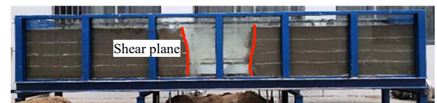
(c) Soil deformation after the 3 rd step of adjustment (complete collapse stage)
