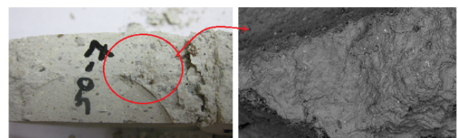
(a) Failure surface and the notch crack tip in the CCNBD specimen and the SEM image
