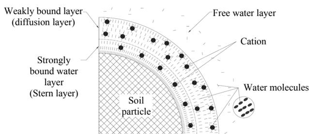
**Fig. 7** Oriented arrangement diagram of bound water molecules
