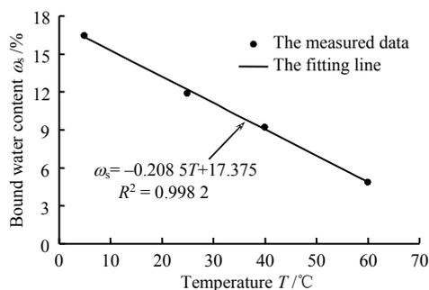
**Fig. 6** Variation curves of bound water content with temperature
