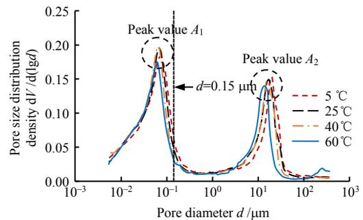
Fig. 5 Curves of pore size distributions under different temperatures
