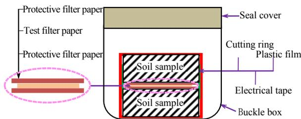
Fig. 1 Sketch of filter paper method
