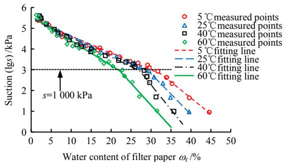
**Fig. 2 Calibration curves of Whatman No. 42 filter paper at different temperatures**
