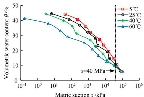
**Fig. 3 SWCCs of Nanning expansive soil at different temperatures (ρ<sub>d</sub> = 1.5 g/cm<sup>3</sup>)**
