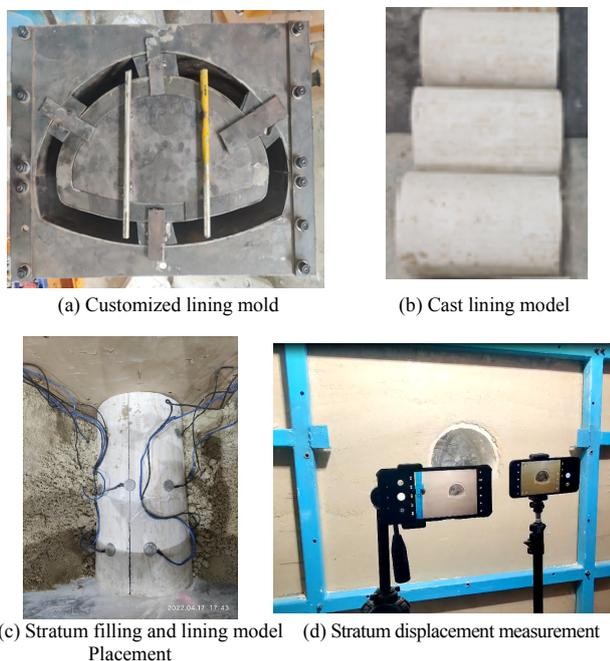
Fig. 6 Implementation of static pushover test
