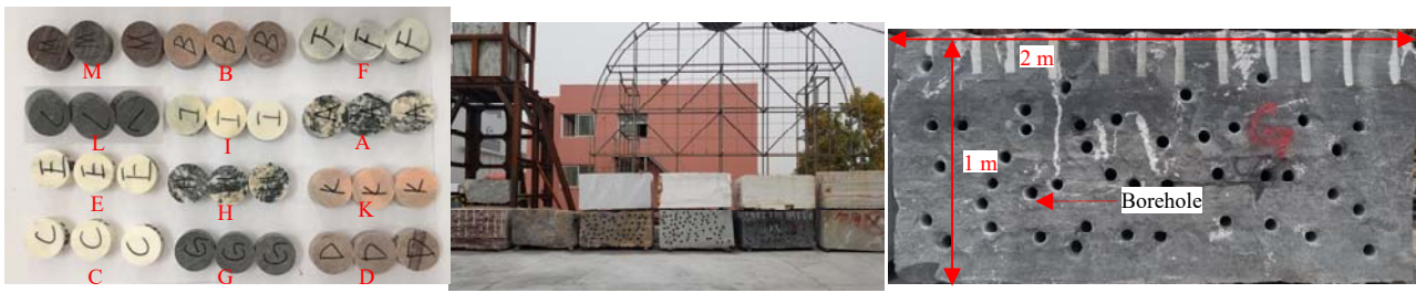
(a) Rock specimens with a diameter of 5 cm (b) 12 rocks with a length, width, and height of 2 m, 1 m, and 1 m (c) Boreholes in percussive drilling tests
