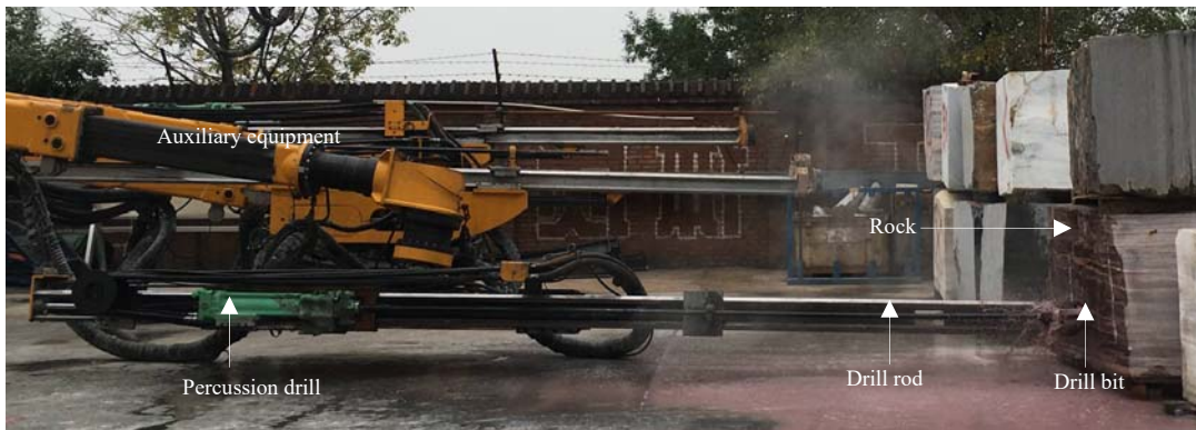
(b) Laboratory tests for percussive drilling
